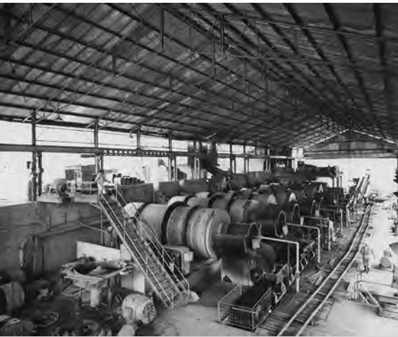
(from left) Ore being scrubbed, rinsed, and loaded onto railcars.
