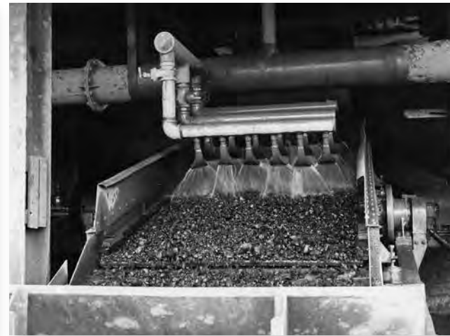
(from left) Ore being scrubbed, rinsed, and loaded onto railcars.
